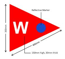
**Figure 4:** Directional signage: fade resistant, fixed to rigid post in contrasting lettering, white sign writing on red background, with a circle reflective marker. 'W' in 150mm upper case lettering.
