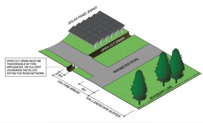
Figure 5: Typical cross-section indicating fire break requirements.
