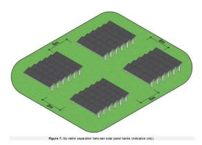
The proposal provides for the 6m separation between solar panel banks.
