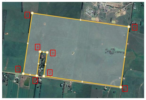
It is important to note that the entire area is not covered with PV panels. To create a more realistic footprint for the purposes of modelling, it is assumed that there is an approximate 15-metre setback from the outside boundaries of the Project with a 15-metre internal setback from the buildings within the site boundary.
